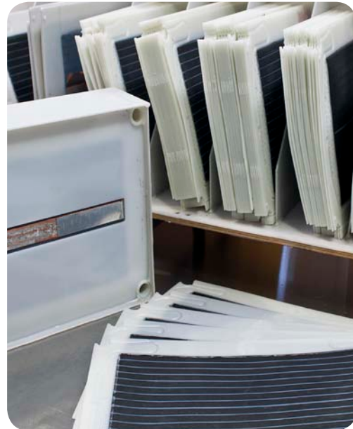
Photo 6. Plastic electrode plates for basic RedFlow ZBM module
