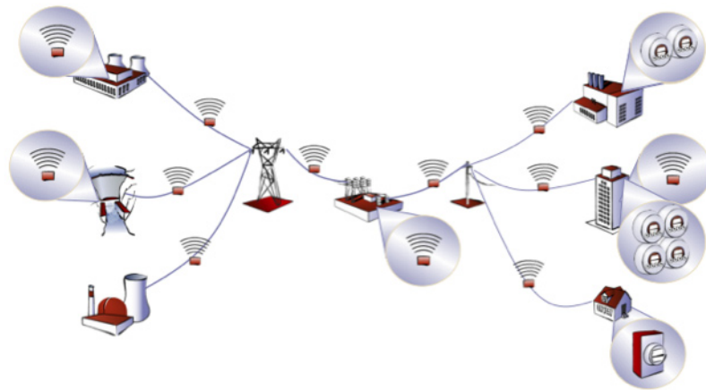
Figure 12: Smart communicating devices can be embedded all along the value chain. They can monitor and dispatch generation; measure voltage, power flow and line sag; report on the condition of expensive transformers; protect vital circuits; meter power; and more.
